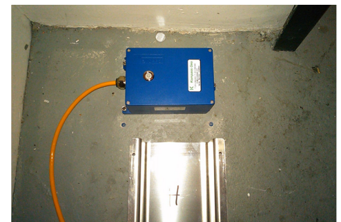
An AC-73 accelerometer in situ.
