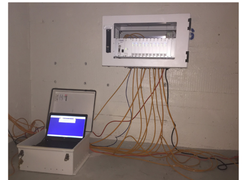
The CR-6plus installed in the Centre Block, ready to record seismic data.
